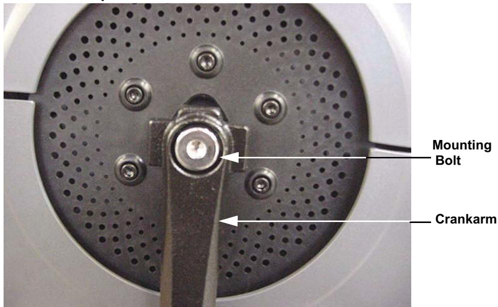
3. Remove the crankarm. It may be necessary to use a gear puller or pitman arm puller to remove the crankarm.
