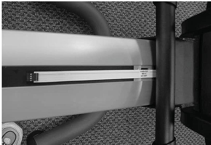
7. Remove the plate that covers the hand held heart rate cable on the bottom of the seat. See Diagram 7.6. The cable may be stuck to the plate with double sided tape.
