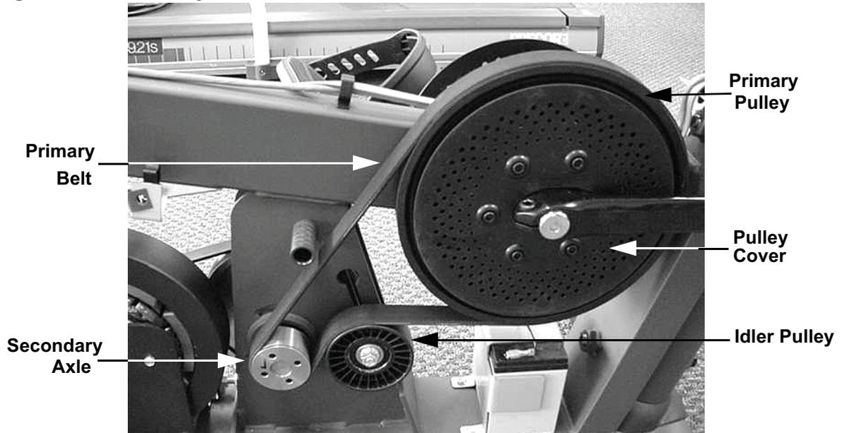
3. Remove the primary belt. Route the replacement primary belt around the primary pulley, over the idler pulley and around the secondary axle as shown in Diagram 7.9.
