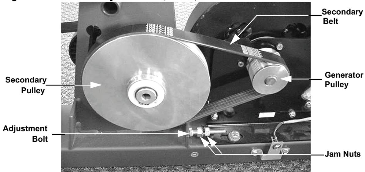
3. Route the replacement secondary belt over the secondary pulley and generator pulley as shown in Diagram 7.10.
