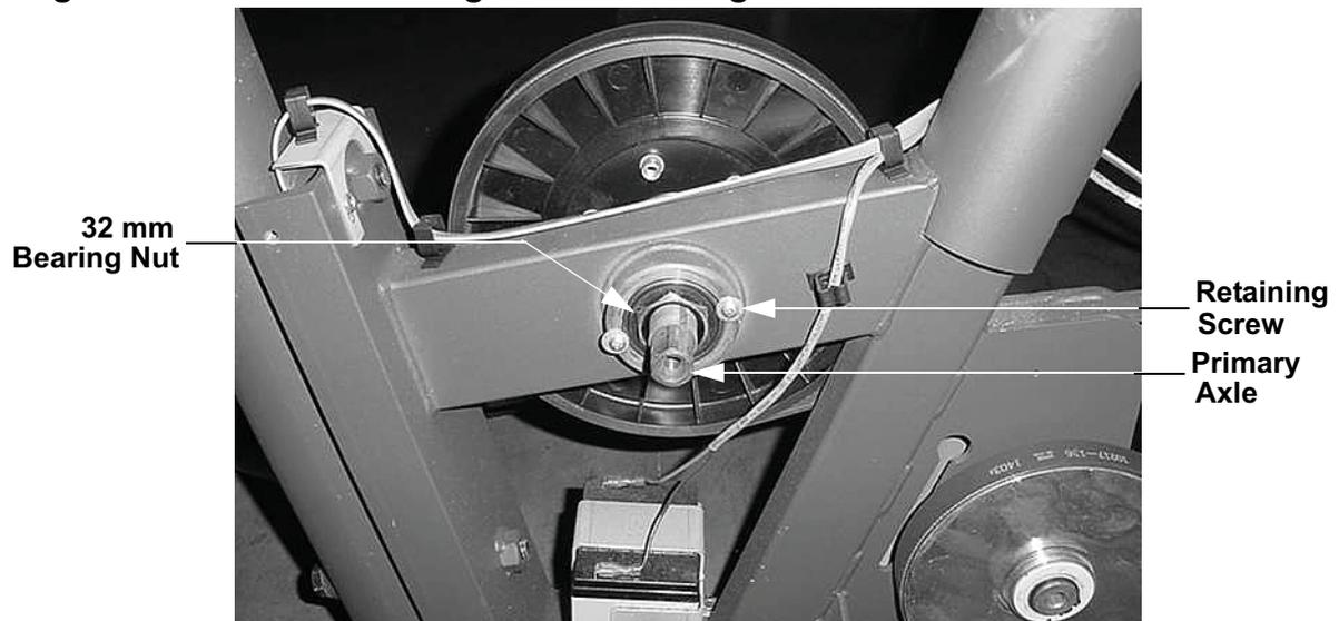
8. Carefully, clean both bearing pockets with a clean dry cloth. You may apply a thin coat of lubricant to the bearing pockets to facilitate re-installation of the bearings.
