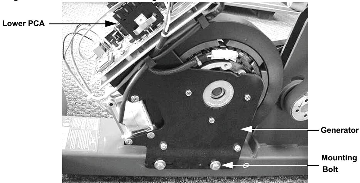
6. Remove the generator with the lower PCA from the bike.
