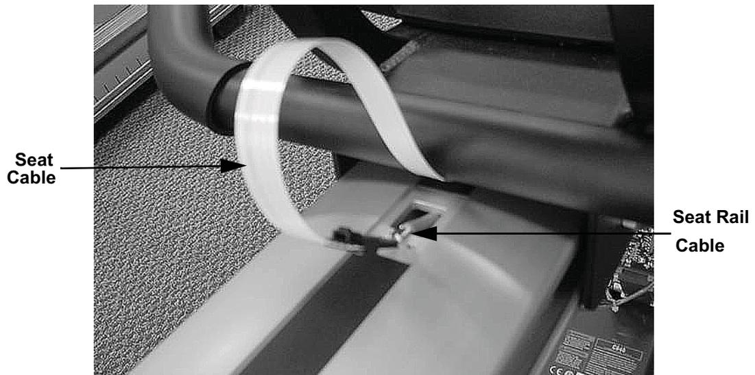
6. Slide the seat rail cable back into the access hole. The seat carriage must travel over this cable, so it must be below the surface of the seat rail. Release the seat lever, hold the cable attached to the seat straight back from the seat as you slide the entire seat and seat carriage off of the rear of the seat rail. See Diagram 7.5.
