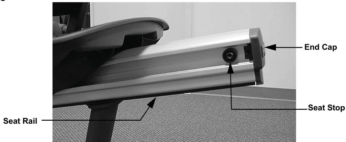
3. Loosen but do not remove the two screws retaining the end cap. Remove the end cap. Remove both seat stops, one each side.
