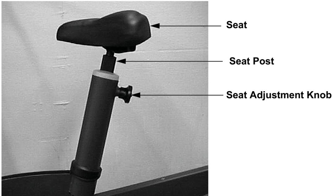
3. Pull the seat adjustment knob outward, slide the replacement seat post into place in the cycle's frame. Release the seat adjustment and move the seat post until the seat post locking mechanism snaps into place and locks the seat post into position.
