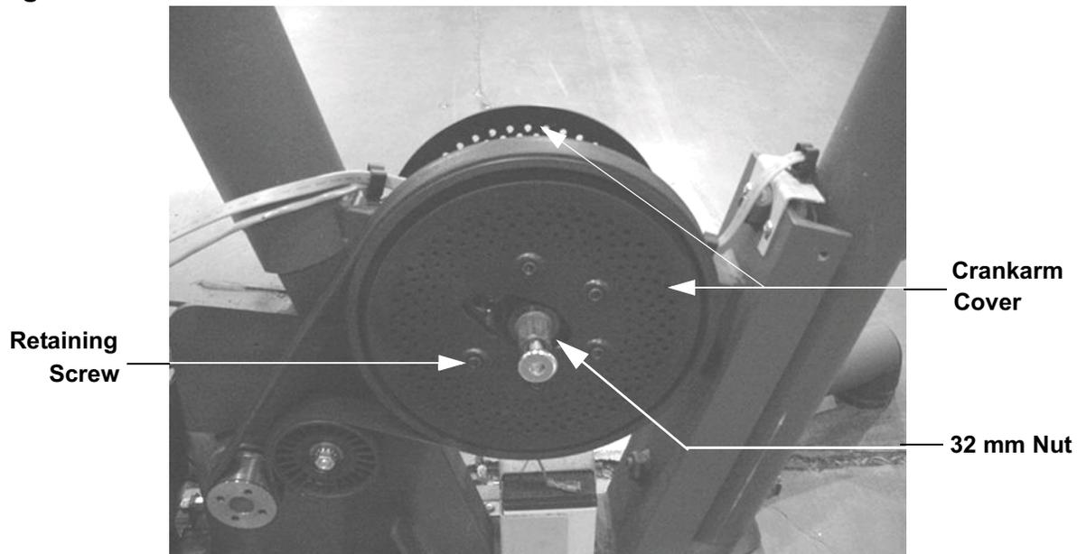
4. Remove the 32 mm nut from the left side of the primary axle. See Diagram 7.12.
