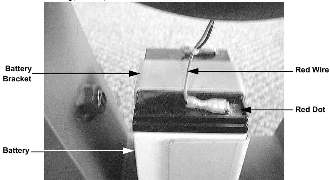
5. Fasten the battery bracket with battery to the frame with the screws removed in step 13.
