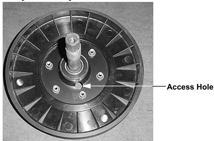
10. Slide the primary pulley assembly into the frame from the right hand side. Slide the left hand bearing over the primary axle and hand thread the bearing nut onto the primary axle. When you are sure the bearing nut is properly threading onto the primary axle, not cross-threading, torque the bearing nut to 60 inch-pounds.
